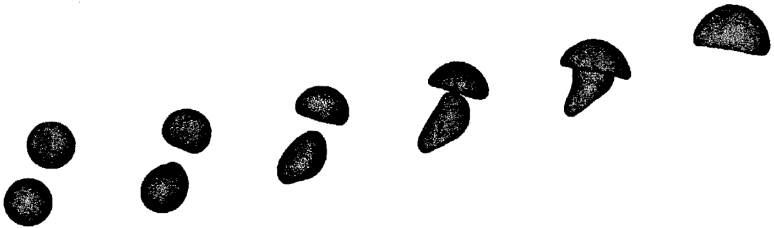
Fig. 16. Transient solution of the bubble coalescence in a continuous phase, the bubbles are not in-line, for t = 0.0 s, t = 0.03 s, t = 0.06 s, t = 0.09 s, t = 0.12 s and t = 0.15 s.
